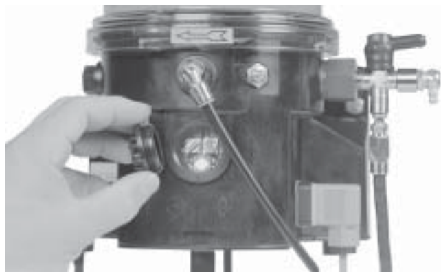
Fig. 12 - The cover to the printed circuit board has been removed
