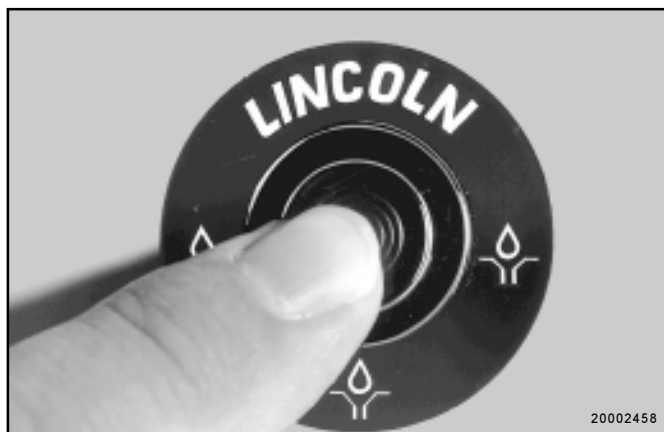
Fig. 21 - External triggering of an additional lubrication
