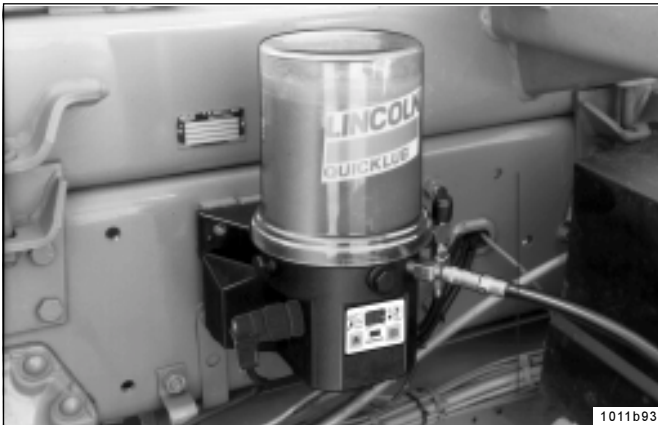
Fig. 37 - Fill pump reservoir
